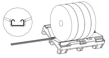
**2.** Insert long channel into slot in bottom of cradle between rolls and pallet
