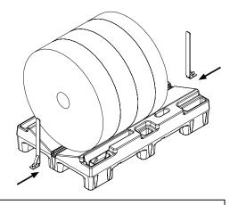
**3.** Insert two black end-pieces into channel on both ends
